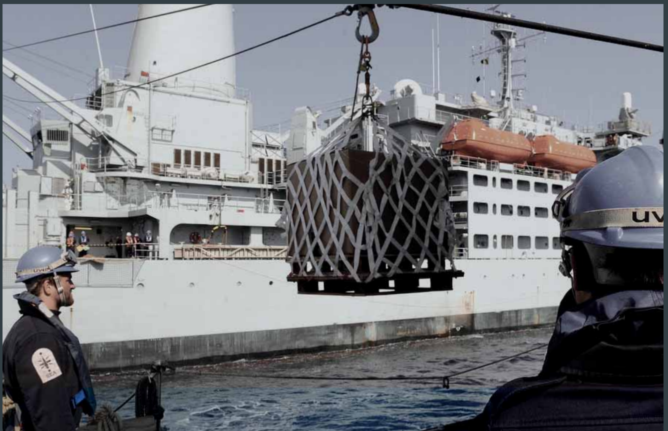
A heavy jackstay in use in 2012. A device of this type was used to transfer nuclear weapons at sea between ships that went to the Falklands
